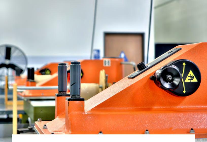
Die cutting is a versatile manufacturing process used to create precise shapes, designs, and patterns on flat, low-strength materials, such as fabric, film, foam, plastic, rubber, sponge, wood, and adhesives. Compared to other production methods, die cutting offers greater precision, complexity, and uniformity, all of which make it ideal for high-volume productions. Typical products range from common household goods and basic office supplies to complex industrial parts and products.
